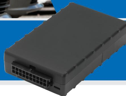
The LMU-2630 fleet tracking unit offers leading edge fleet management features including a triple-axis accelerometer for measuring driver behavior and vehicle impacts while offering the high reliability fleet customers demand.
